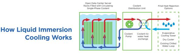
Heated coolant exits top of rack. Coolant returns to rack from heat exchanger at user-specified temperature.
